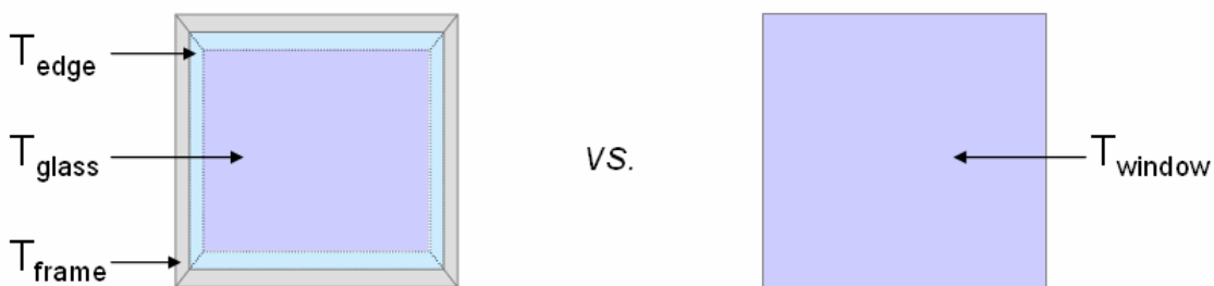
Figure 28: Explicit modeling of window components vs. uniform window temperature
