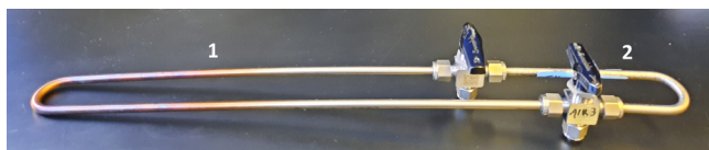
Figure 2. Molecular sieve trap with two three-way valves. Part 1 holds the molecular sieve in the bottom secured by quartz wool. Part 2 is a bypass to flush the system prior to sampling.
