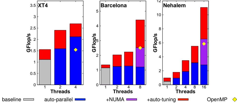
**Figure 2.** Laplacian performance as a function of auto-parallelization and auto-tuning. For comparison, the yellow diamond shows performance achieved using the original stencil kernel with OpenMP pragmas and NUMA-aware initialization.
