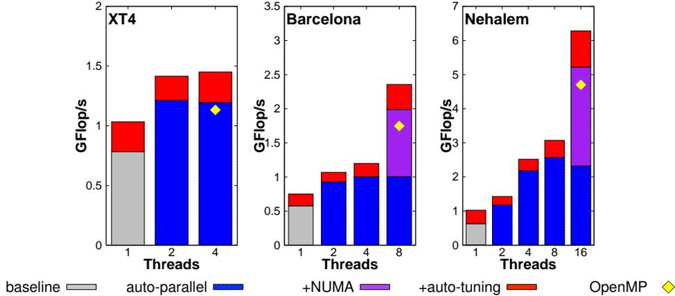
**Figure 3.** Divergence performance as a function of auto-parallelization and auto-tuning. For comparison, the yellow diamond shows performance achieved using the original stencil kernel with OpenMP pragmas and NUMA-aware initialization.
