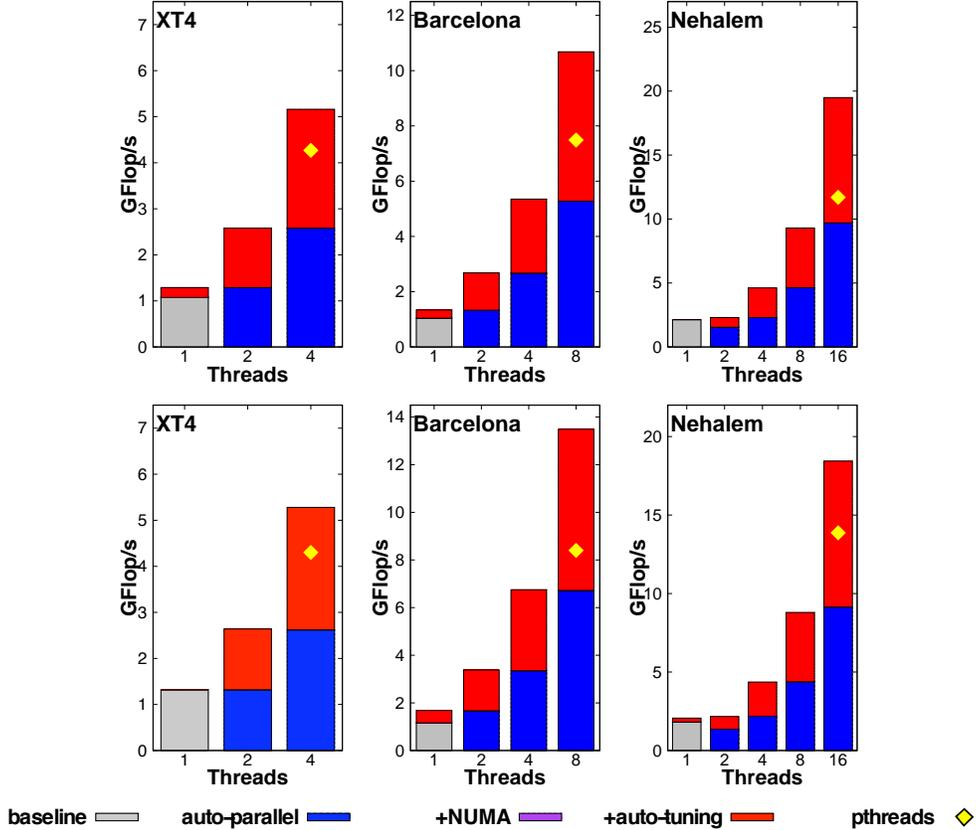
**Figure 5.** Bilateral filtering performance as a function of auto-parallelization and auto-tuning, for radius 3 (top) and radius 5 (bottom). For comparison, the yellow diamond shows performance achieved using a handwritten pthreads filtering implementation with NUMA-aware initialization.
