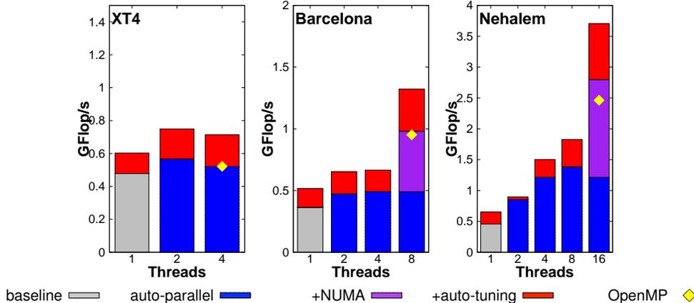
**Figure 4.** Gradient performance as a function of auto-parallelization and auto-tuning. For comparison, the yellow diamond shows performance achieved using the original stencil kernel with OpenMP pragmas and NUMA-aware initialization.
