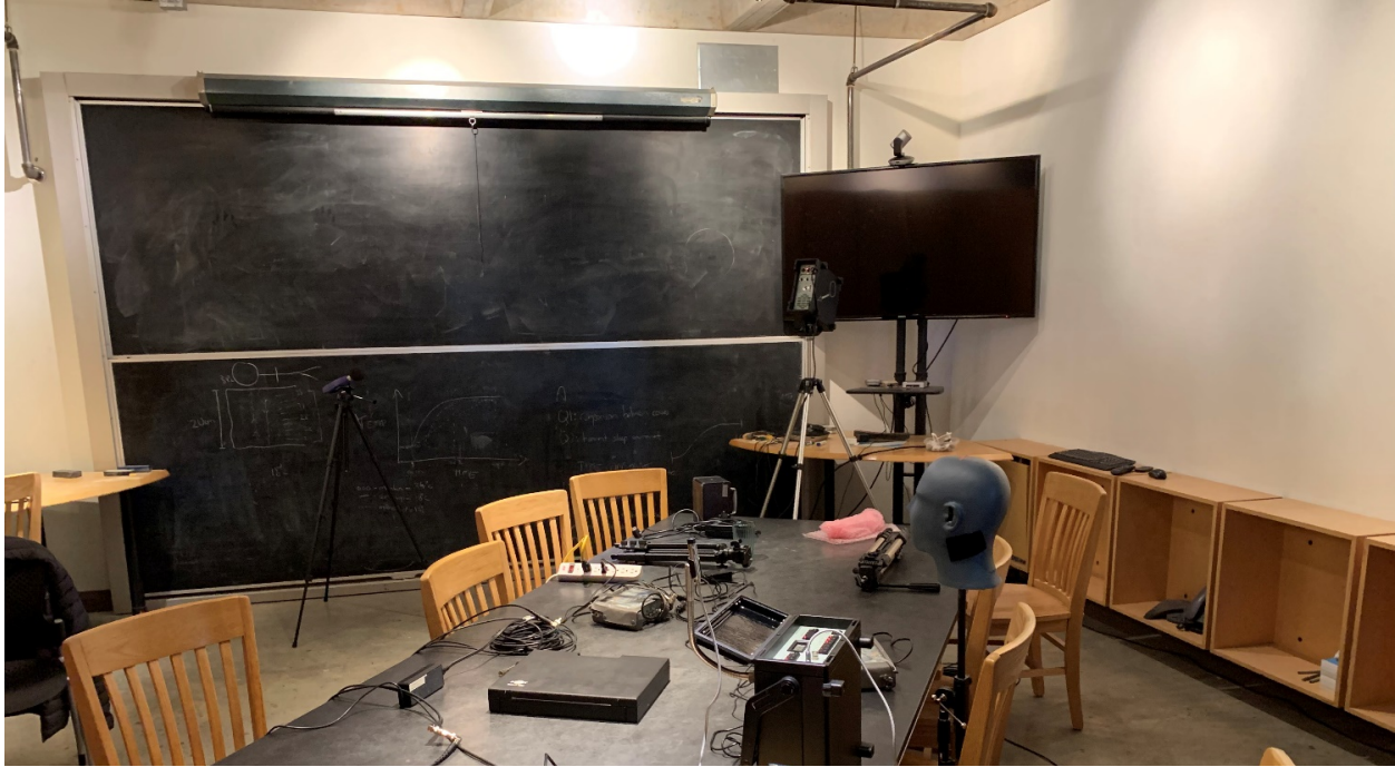
Figure 5: Photograph showing the general layout of measuring instrumentation in Room 390. A sound level meter is installed on a tripod close to the left side of the blackboard. The device on the silver tripod to the right is the transmitter portion of a specialized RASTI system (see Appendix 2). The companion receiver portion of the RASTI system is on the table in the foreground. The dark blue manikin head can be seen next to the right side of the table. Additional instrumentation can also be seen in Figure 4 on page 7.
