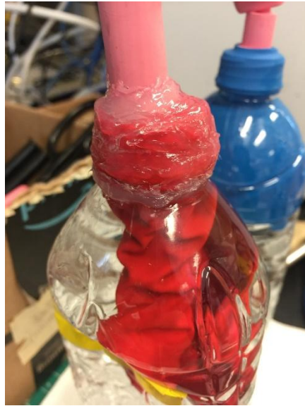
Figure 2.7: Experimental setup with the red and blue balloons containing ferrofluid and a straw, which acts as a guide to flow into the thin pink animal balloon. The water bottle is filled with water, creating pressure onto the balloon when squeezed.
