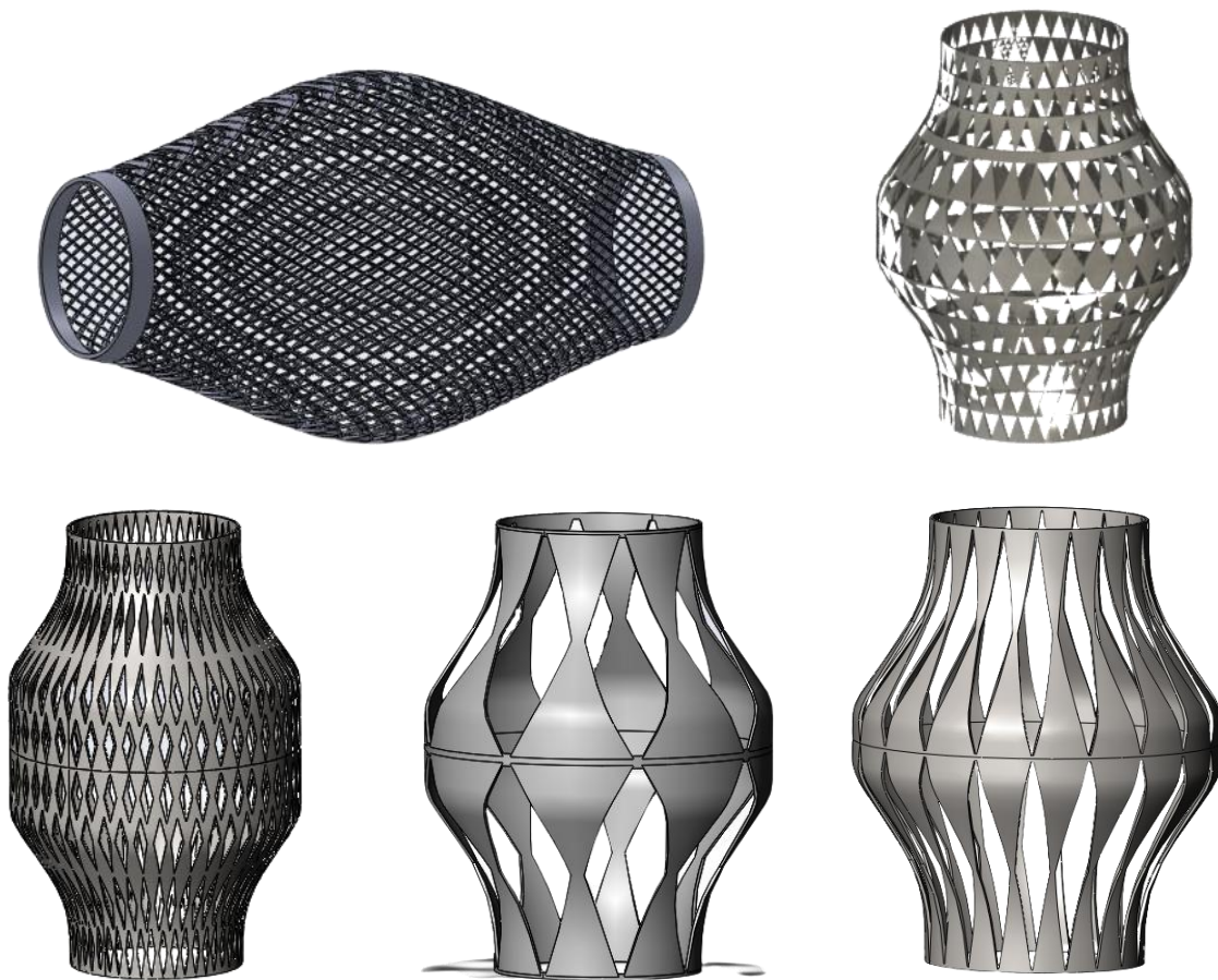
Figure 3.6: a) Various stent cutout geometries tested to find the optimal pattern shape.
