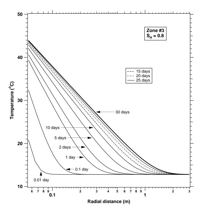
Fig. 11. Temperature distribution during thermal dissociation of hydrates in Zone #3.
