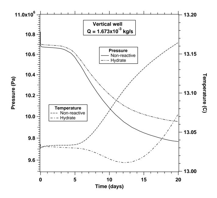
Fig. 2. Evolution of pressure and temperature at the vertical well in Zone #1.
