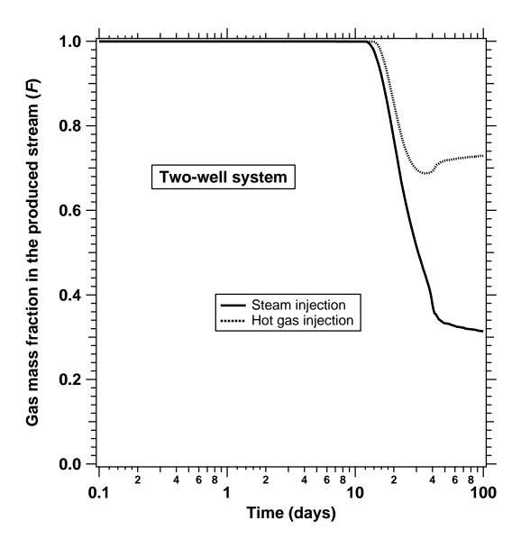
Fig. 6. Gas mass fraction in the production stream of the two-well system in Zone #1.
