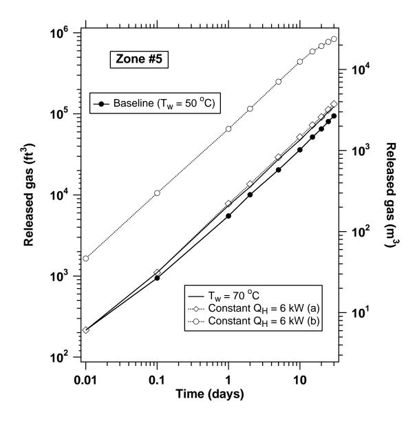
Fig. 16. Sensitivity of gas production to the method of heat addition and to the well boundary conditions.
