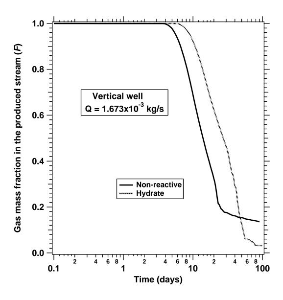
Fig. 3. Gas mass fraction in the production stream of the vertical well in Zone #1.
