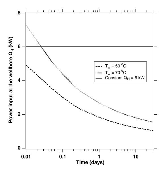
Fig. 17. Power addition  $Q_H$  at the well for the different heating schemes.
