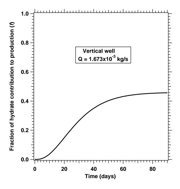
Fig. 4. Hydrate contribution to gas production stream in Zone #1 (vertical well).
