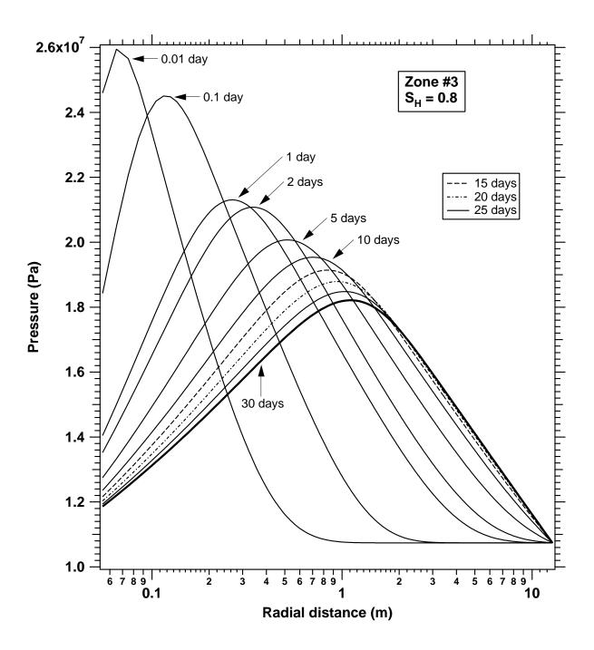
Fig. 10. Formation pressure during thermal dissociation of hydrates in Zone #3.
