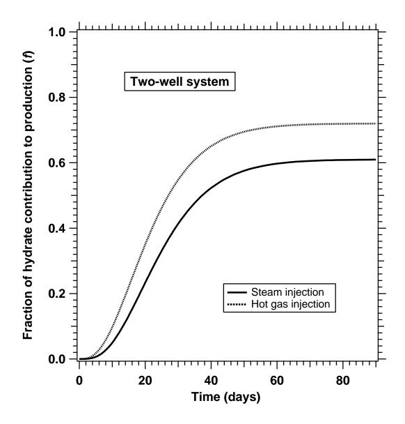
Fig. 7. Hydrate contribution to gas production stream of the two-well system in Zone #1.
