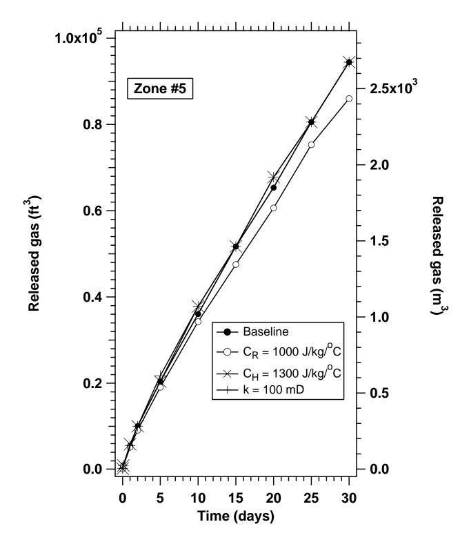
Fig. 18. Sensitivity of gas production to the formation intrinsic permeability k, rock specific heat  $C_R$  and hydrate specific heat  $C_H$ .
