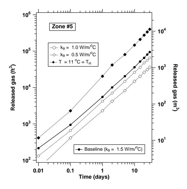
Fig. 15. Sensitivity of gas production to the thermal conductivity  $k_{\theta}$  and to the hydrate initial temperature T.
