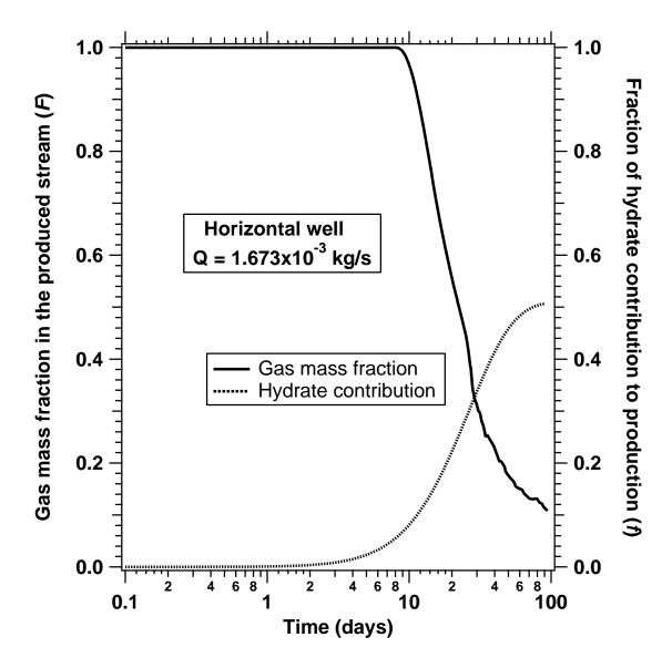
Fig. 5. Gas mass fraction in the production stream and hydrate contribution to gas production stream in Zone #1 (horizontal well).
