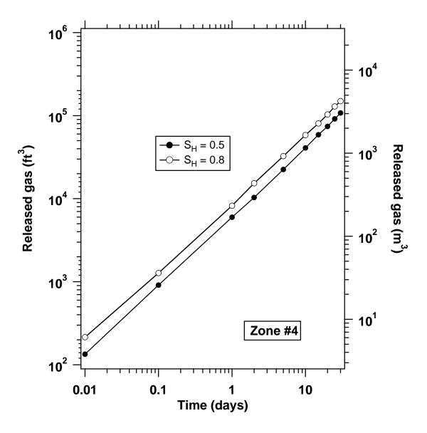
Fig. 14. Sensitivity of gas production to  $S_H$  in Zone #4 (volumes in standard conditions).
