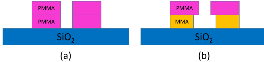
Figure 2.6: The comparison between using PMMA/PMMA and MMA/PMMA as e-beam lithography resist layers. Since MMA is more sensitive to e-beam exposure, more MMA will be washed away after develop. The space will be filled up with metal after metal evaporation, and the extra metal in MMA will act as an anchor point to secure the metal to stay on the wafer.
