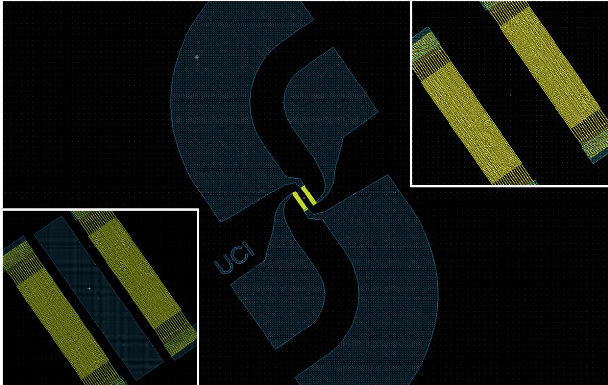
Figure 5.9: **Initial NR-SAW device layout.** Where  $A = 24 \mu\text{m}$ ,  $p = 125 \text{ nm}$ ,  $w = 125 \text{ nm}$ ,  $\lambda_0 = 450 \text{ nm}$ , off- $Z$  angle  $\theta = 35^\circ$ , and IDT separation  $d = 12 \mu\text{m}$ . The lower left inset shows the center zoomed in with the active region SAF included and the top right inset shows the center zoomed in without the SAF. The device was rotated  $35^\circ$  to try and observe the effect with little rotation needed for the chip.
