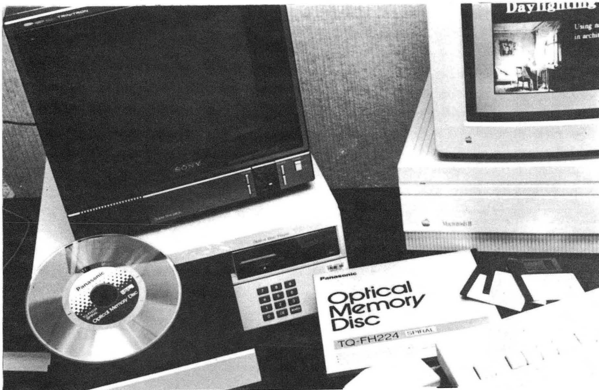
Fig. 5. The workstation today, with 8-inch analog optical disks, magnetic data disks, optical disk player, color video monitor, and microcomputer. Future additions: CD-ROM data storage, digital optical storage, CD audio, and access to central network system. (XBB 894-3731)
