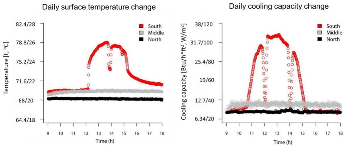
Measured floor surface temperatures at 3 locations: south (near window), middle and north; measured floor cooling capacity at 3 locations.
