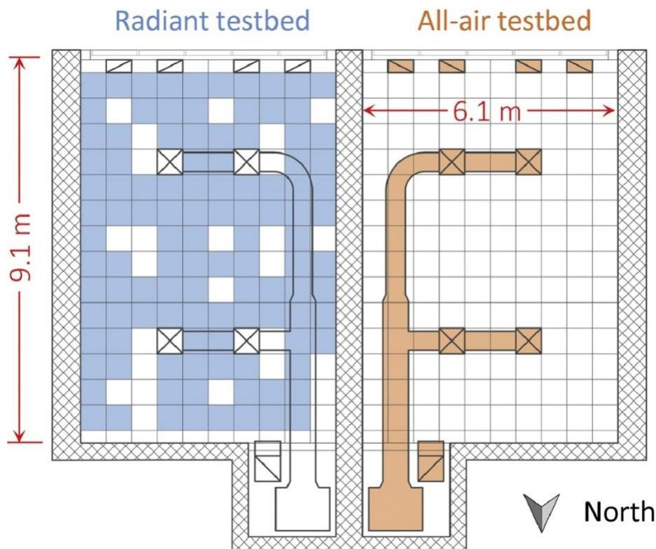
Air handler, overhead ductwork, supply diffusers, and return registers in the all-air testbed are highlighted in orange. Low thermal mass metal ceiling panels in the radiant testbed are highlighted in blue.
