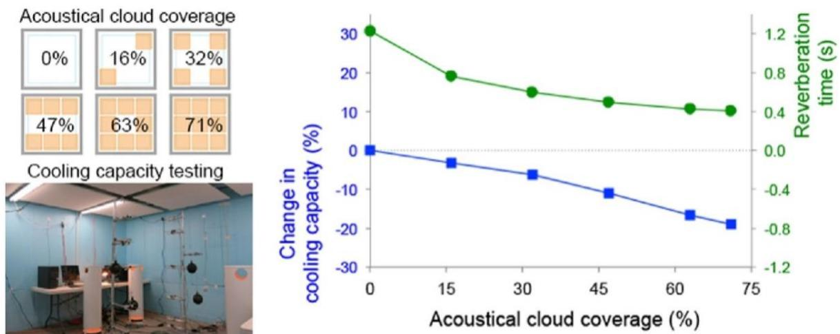
Schematic of acoustical cloud coverage; photograph of laboratory test chamber; measurement results of cooling capacity and reverberation time as a function of acoustical cloud coverage.
