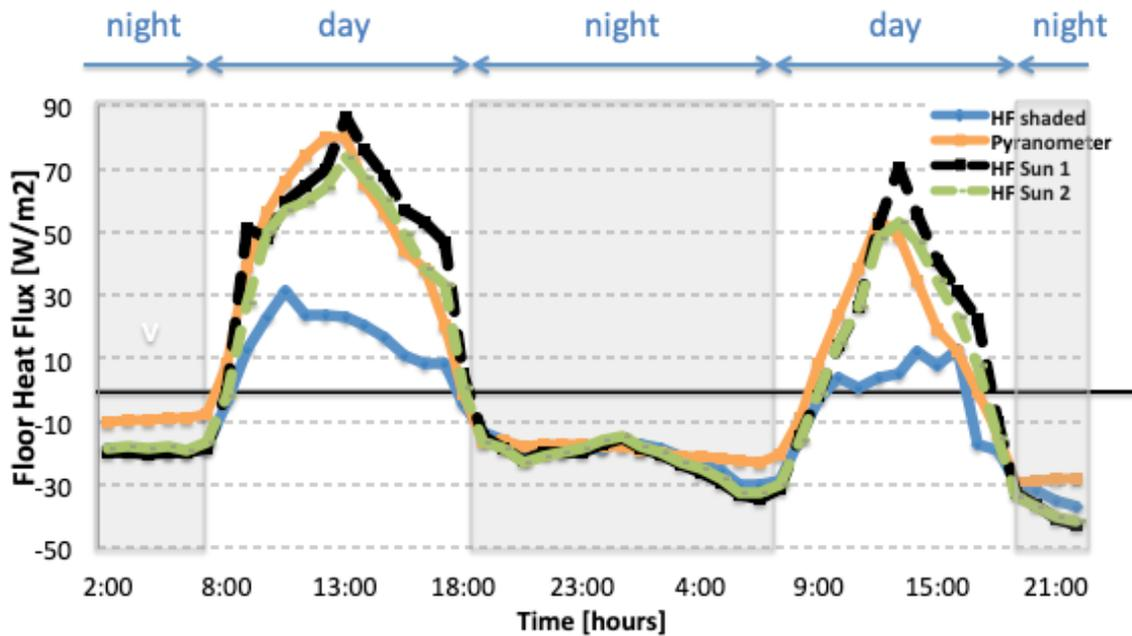
Radiant floor exposure and heat flux in the shaded and sun-exposed regions; Oct. 19-20, 2016.
