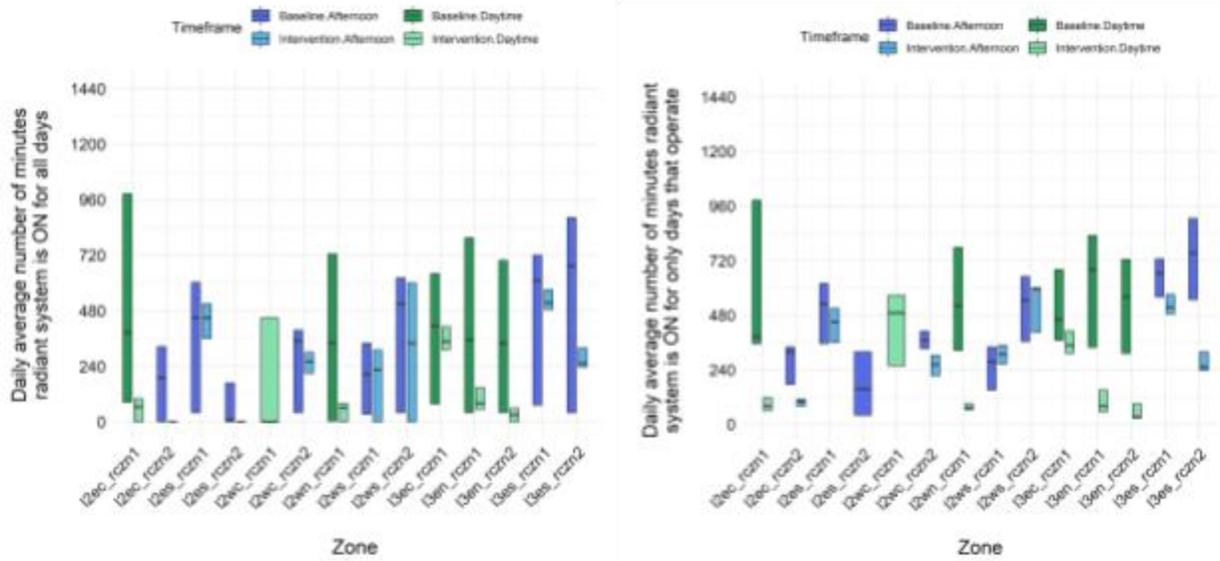
Daily number of minutes that radiant system is actuating the manifold valve in each radiant zone to ON, during all days in dataset (left) and only for days when the manifold turned ON (right).
