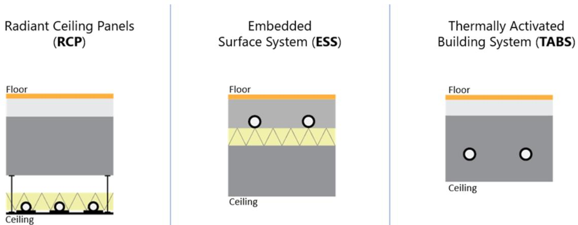
In terms of cooling in California climates, radiant slab systems can take advantage of the high thermal mass of the slab to significantly reduce peak cooling loads and allow structural pre-cooling strategies to be implemented during nighttime hours when both utility rates are lower and ‘free cooling’ can be achieved due to lower outside dry and wet-bulb temperatures. Overall, this can substantially reduce the required size of system components.
