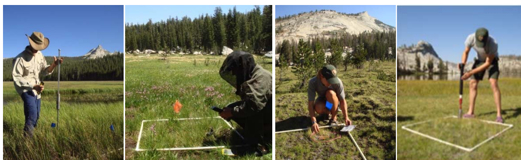
Figure 4. Stratified random sampling with 1 m 2 study plots (quadrats). In-situ sampling done for following: soil resistance (using dynamic cone penetrometer; far left), soil moisture (using TDR; middle left), absolute aerial foliar cover (via ocular estimation; middle right), and soil sampling (using AMS corer; far right).
