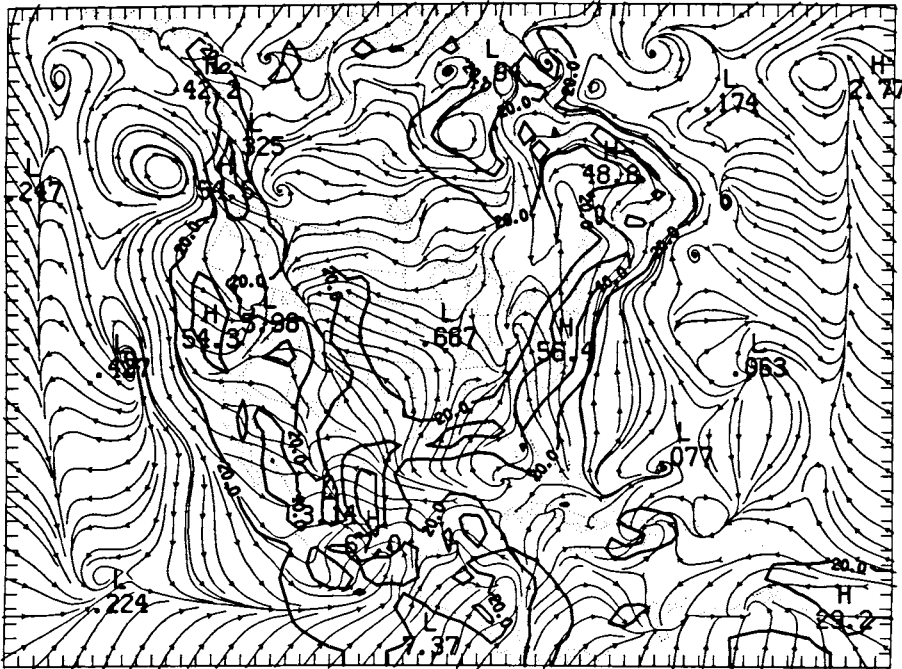
Figure 4. Streamlines (thin lines) and isotachs (heavy lines in m s^{-1} times 5) in the boundary layer ( \sigma = 0.95 ) at 72 h of Exp. 1.
