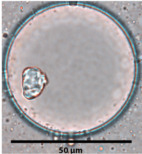
Figure 79. Successful cellulose particle encapsulation within an emulsion droplet. Solid particles had not been encapsulated with IVC emulsions previously.
