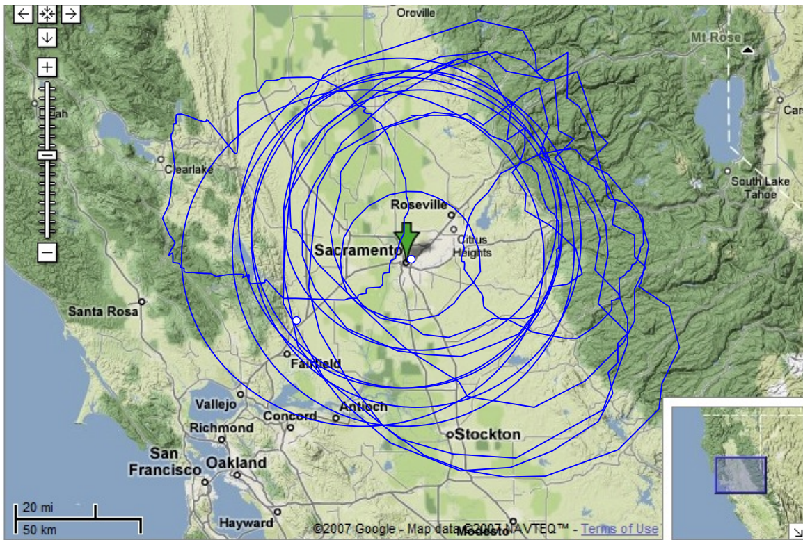
Figure 4. Local signal coverage for FM Stations sending RDS signals. Signal coverage data from the Federal Communications Commission.
