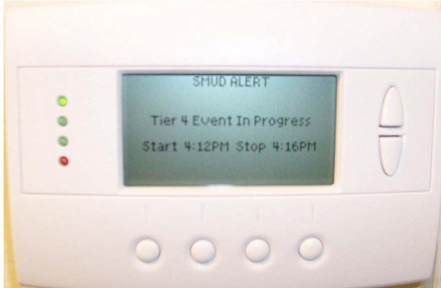
Figure 25. PCT displaying Tier 4 event in progress
