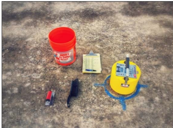
Figure 3.3: Soil stiffness gauge.
