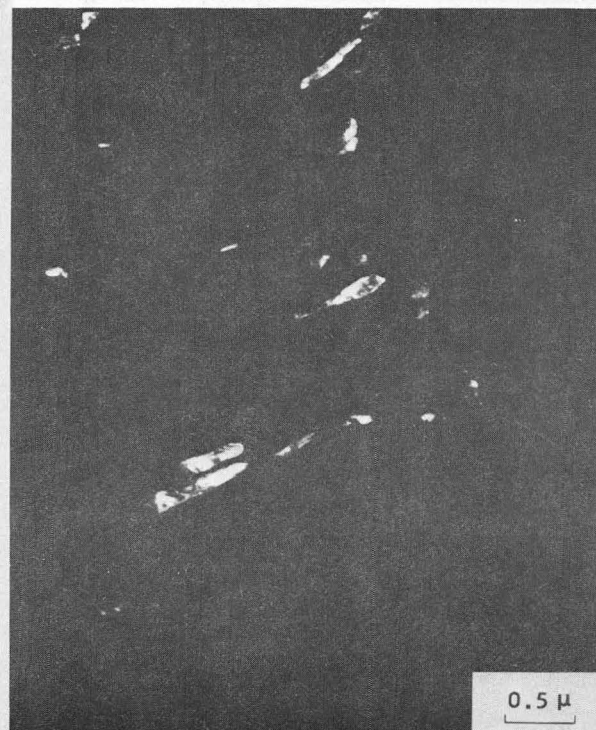
Fig. 5 - Electron diffraction analysis of retained austenite in a specimen heat treated at 600°C after grain refinement.
