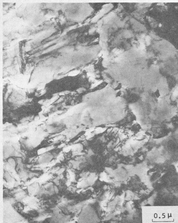
Fig. 5 - Electron diffraction analysis of retained austenite in a specimen heat treated at 600°C after grain refinement.
