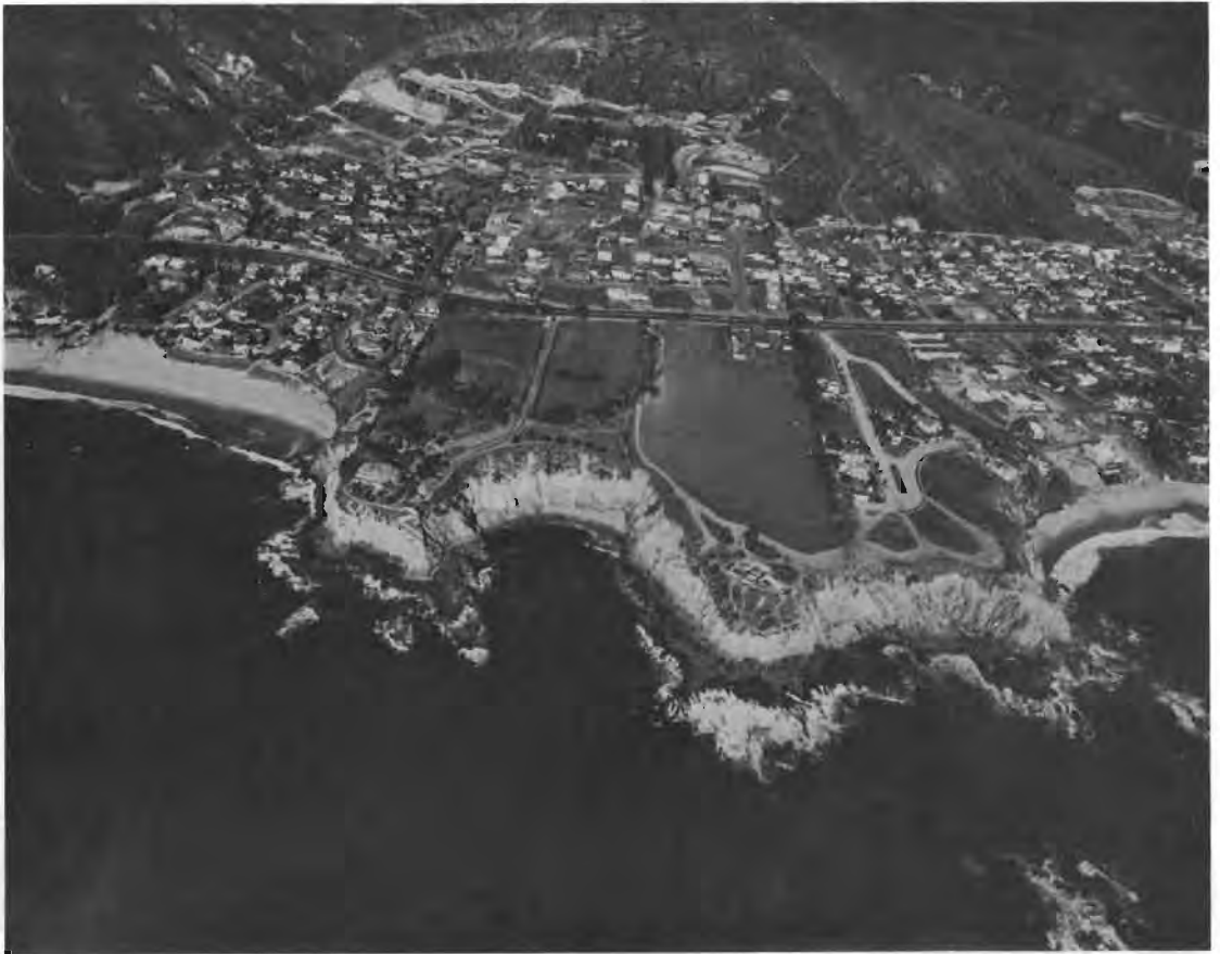
Figure 7. Laguna Beach. Cliffs consist of Miocene schist breccia and basalt. The marine terrace is between 80 and 120 feet above sea level. At the base of the cliffs is a low rock terrace of the type sometimes known as a storm terrace. Note the pocket beaches, only one of which is at the mouth of a stream. Photographed by R. E. Stevenson in 1952.
