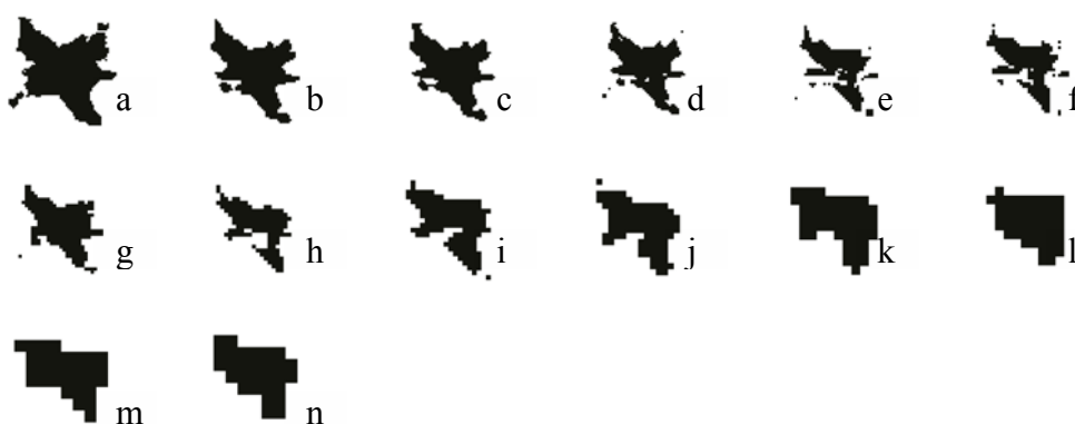
Figure 2. Shrubs representations at different spatial resolutions ranging from 9.13 mm (a) through 54.75 mm (n).
