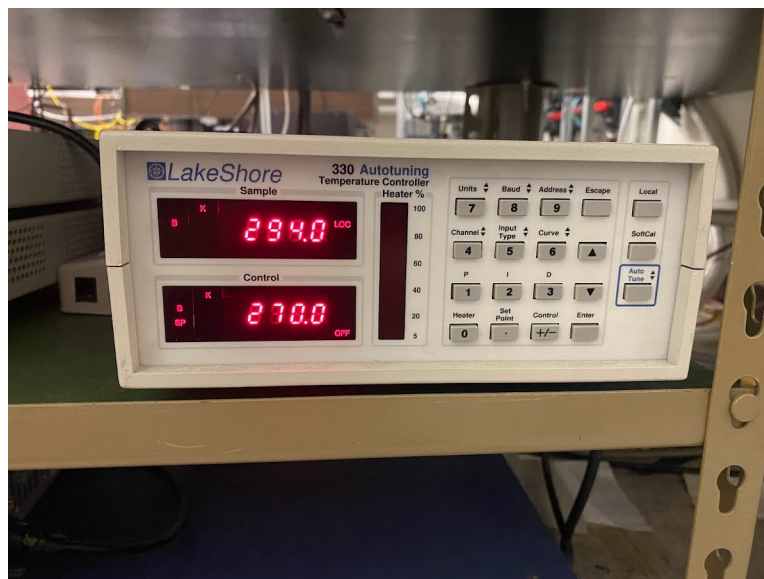
Figure A.6: Temperature controller. The LakeShore 330 temperature controller. The top left display shows the measured temperature, and the the bottom left display shows the set temperature. When heating is active, the percentage of heater power is shown on the right.
