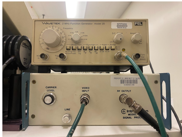
Figure A.4: AOM driver and function generator. Top: The Wavetek function generator used to trigger the AOM in quasi-CW mode. We use a square wave of roughly 100 kHz for a functionally CW NIR signal. Note that because this is a square wave the NIR will have a 50% duty cycle and any measured power will be half of the true power. Bottom: The AOM driver. The driver is turned on by pressing the line button, and the carrier level controls the strength of diffraction. At zero, no signal transmits through the system. At ten, maximum strength transmits. Put the electronic signal on the video input BNC connector. This signal is either from the function generator or the delay generator. The RF output connects the driver to the AOM.
