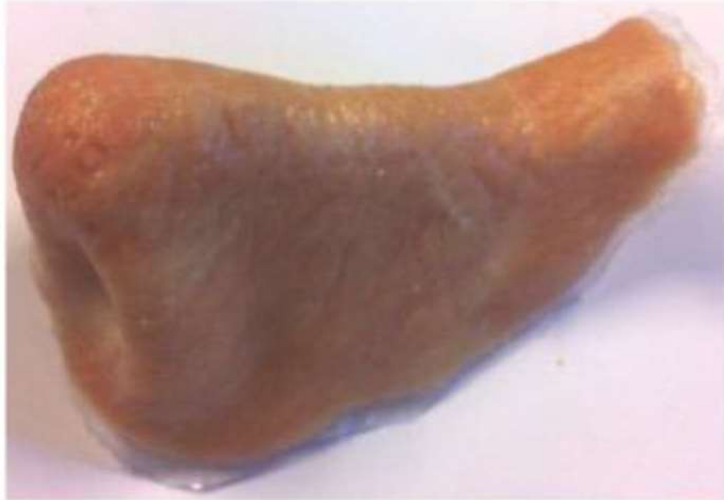
Figure 1-13. Nasal Prostheses fabricated based on Binder Jetting Approach. Reproduced with Permission from [24].
