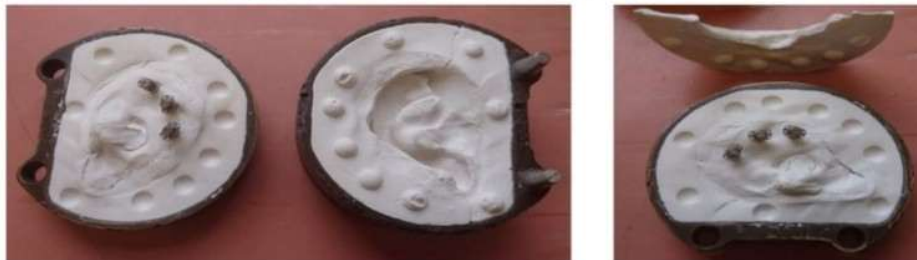
Figure 1-2. (a-d) Digital Based Ear Replica and Mold Fabrication processing for Maxillofacial Prostheses. Reproduced with permission from [9].
