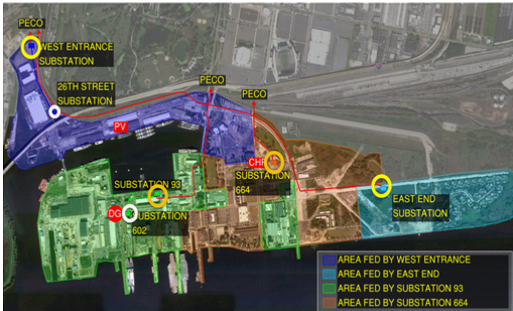
Figure 3.11. TNY Distribution grid overview with substations
