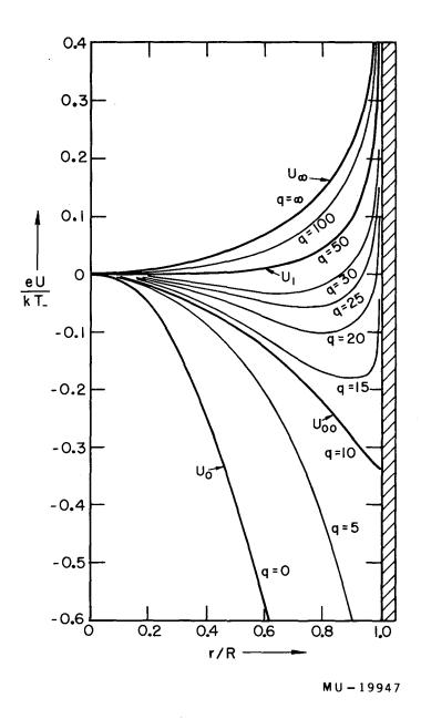
Fig. 3. The ambipolar radial potential distribution is plotted as a function of the relative radial distance r/R. The parameter values are identical with those in Fig. 2.
