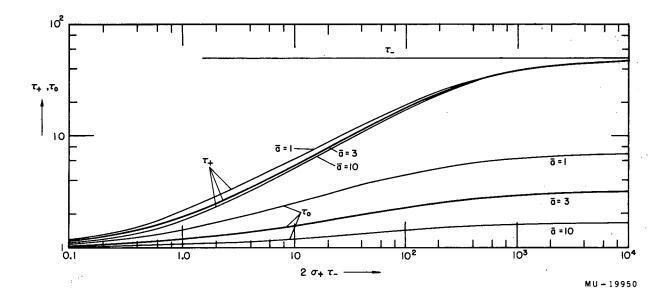
Fig. 6. This figure gives the relative ion  $(\tau_+)$  and gas  $(\tau_0)$  temperatures (see eq. 80) as a function of the enhancement parameter  $2\sigma_+\tau_-$  for three values of a (see eq. 87) and a constant electron temperature  $\tau_-=50$ .
