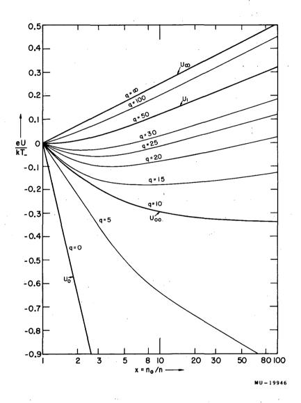
Fig. 2. This figure gives the ambipolar radial potential distribution (U) as a function of the density ratio  $x = n_o/n(r)$  for parameter values of  $q = u_+u_-B^2$  in the range  $o \rightarrow \infty$ .  $-\sigma_{o-} + \sigma_{o+} = 5 \cdot T_-/T_+ = 10.$
