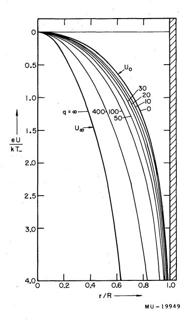
Fig. 5. The radial potential distribution (U) for Simon diffusion plotted versus the relative radial distance r/R. All conditions are identical with those of Fig. 3.
