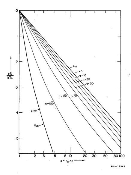
Fig. 4. The radial potential distribution for Simon diffusion (U) is given as a function of the relative density  $x = n_0/n(r)$ . The parameter values are identical with those stated in Fig. 2. In addition we have  $\mu_{-}/\mu_{+} = 10^{2}$ .
