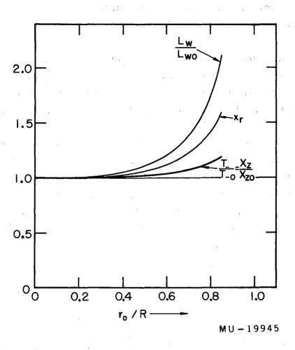
Fig. 1. This figure shows  $x_r$ , the solution of eq. (15) normalized to unity at  $r_0 = 0$ ;  $L_w/L_{wo}$ , the relative wall loss;  $T_-/T_{-0}$ , the relative electron temperature; and  $X_z/X_{z0}$ , the relative longitudinal electric field as functions of  $r_0/r$ . Here  $r_0$  limits the region of enhanced diffusion  $(D_{\perp} \rightarrow \infty)$ , R is the radius of the discharge tube.
