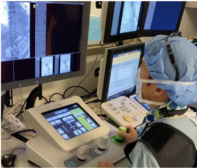
Figure 3 Catheter manipulation using a push–pull and rotation joystick control solely based on the visual information.
