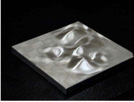
FIGURE 9. MACHINED SURFACE USING 0.25IN DIAMETER CUTTER.
