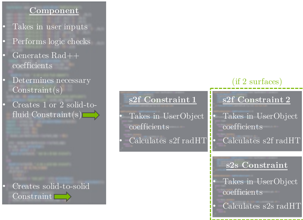
Figure 3.4: RadiativeHeatTransfer code framework showing component for interfacing with user and constraints called for Rad++ calculation.
