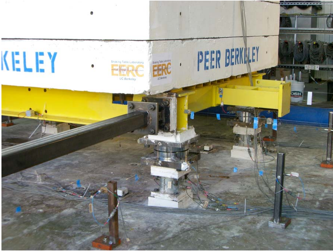
Figure 3.5 View of instrumentation surrounding the TFP bearing
