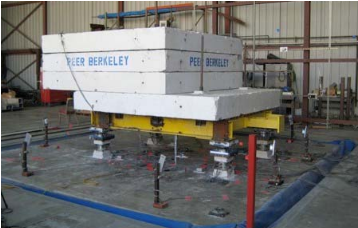
Figure 4.22 Rigid block experimental setup with offset center of mass at the UC Berkeley Earthquake Simulator Laboratory
