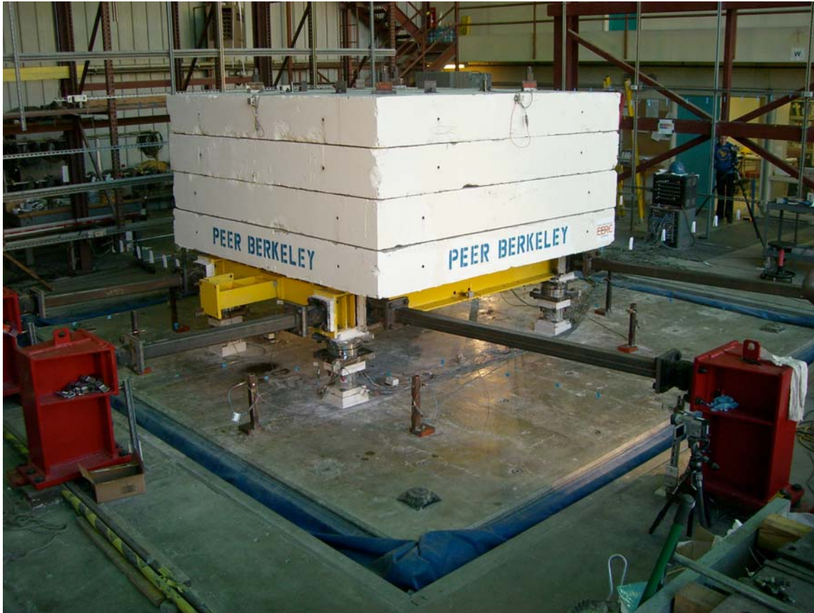
Figure 3.3 Rigid block experimental setup at the UC Berkeley PEER Earthquake Simulator Laboratory
