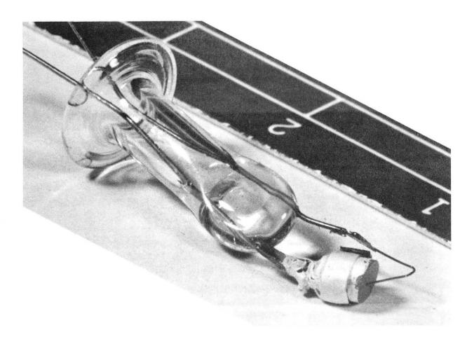
Fig. 13. A barium titanate lamp without the outer glass envelope. The scale is graduated in centimeters.
