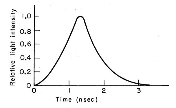
Fig. 10. Corona lamp light-pulse shape.
