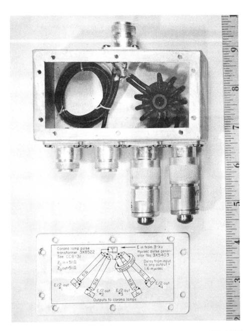
Fig. 7. Pulse splitting transformer.
