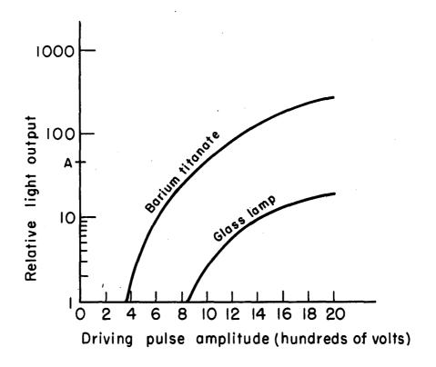
Fig. 12. Light intensity as a function of pulse voltage.
