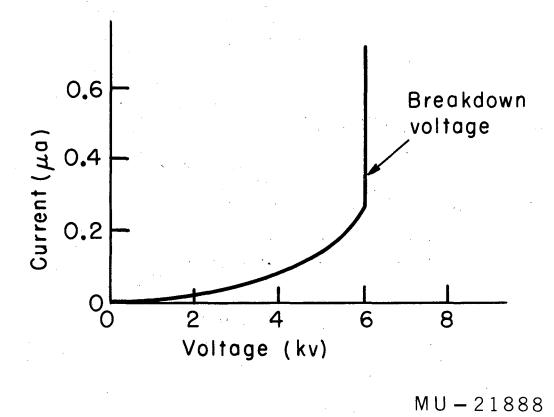
Fig. 3. Typical current-voltage curve characteristic for mercury capsule.
