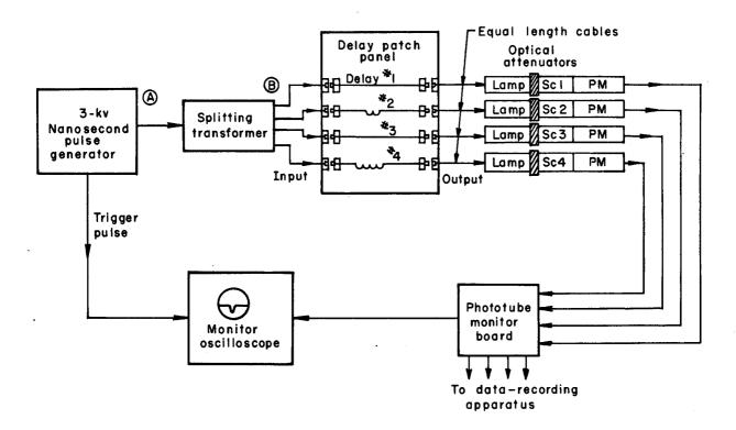
Fig. 1. Corona lamp simulation of a nuclear event.
