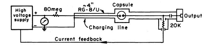
Fig. 4. 3 kv nanosecond pulse generator simplified schematic.
