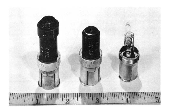
Fig. 9. Photograph of corona lamps. Lamp on the left has the adjustable polaroid attenuator attached.
