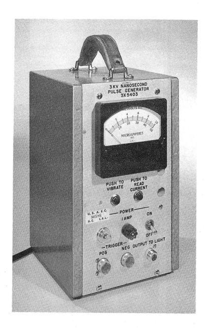
Fig.6. 3 kv nanosecond pulse generator.
