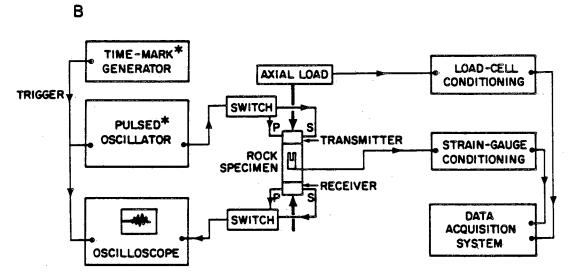
\*Replaced by PUNDIT ultrasonic tester
