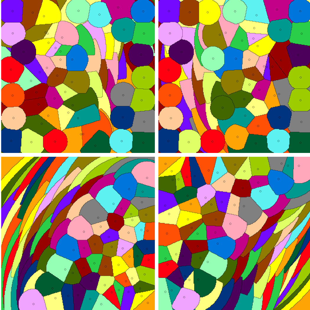
Figure 7.11: Top: Two consecutive iterations of the stable k -means method with weighted centroids for p = 1 , for the same matching from Figure 7.8 with n = 300 and 50 random centers. Bottom: same for p = 10 .
