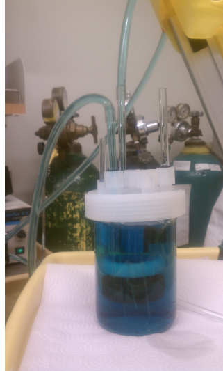
Figure 12: Mixing test for approximately 1L of water. In this photograph, you can see that the blue dye has dispersed homogeneously throughout the 1L beaker. Similar tests were also performed within the 2L vessels used in experiments.
