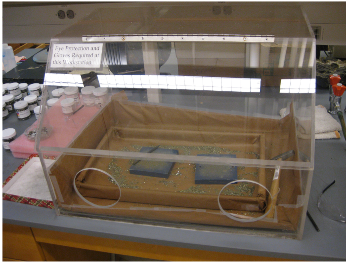
Figure 3: Crushing station with hammer and chisel inside a protective box.
