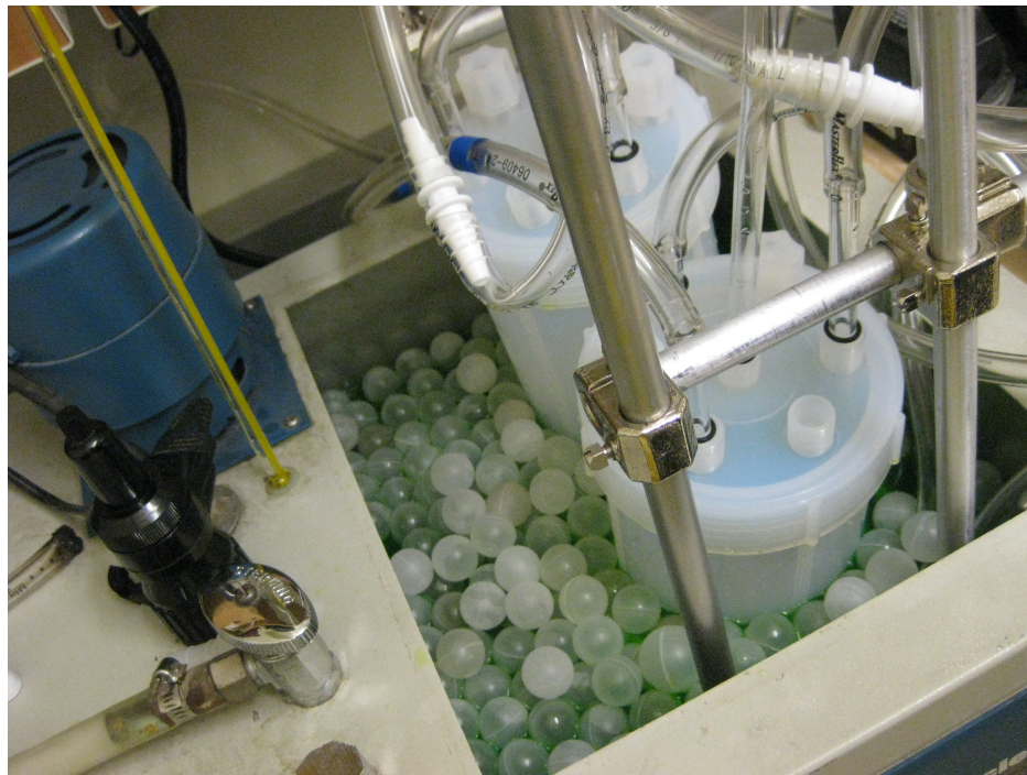
Figure 10: Two 2-liter Teflon reaction vessels sit inside a temperature-controlled bath. The green liquid inside the bath is antifreeze while floating Teflon balls act as insulation. Antifreeze was used instead of water to prevent corrosion of the steel baths.
