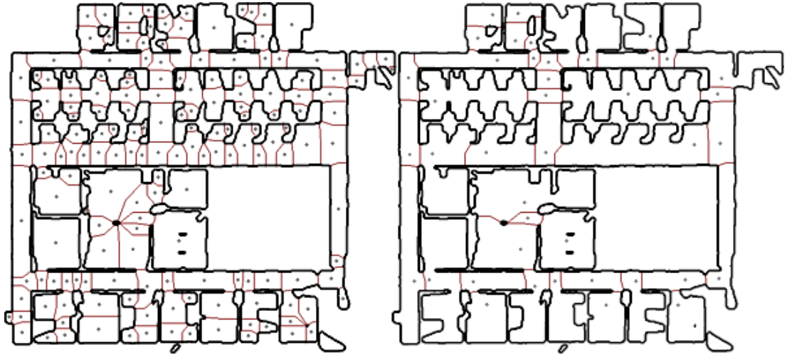
Figure 5.9: The sdr_site.b from Radish [HR03] with initial graph construction. The thick black lines are boundaries between free and occupied space. The small black points are vertices placed in their corresponding region which are separated by thin lines. On the right is final graph resulting from contractions.
