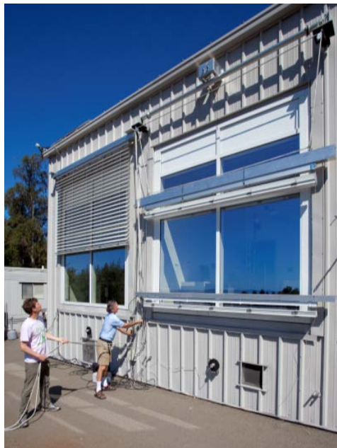
Figure 25: Exterior view of LBNL Advanced Windows Testbed with exterior shading systems
