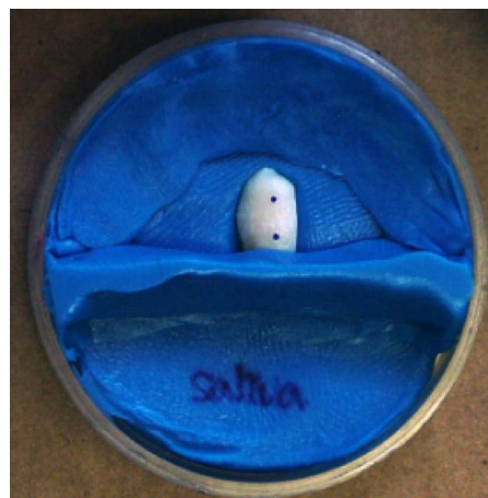
Fig. 1 Sample preparation. Teeth set in silicone mold for OCT imaging. Two oil ink markers indicate the area for imaging.
