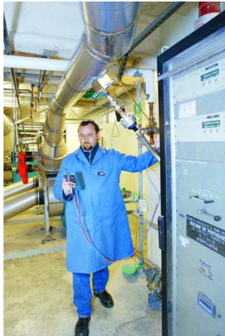
Calibration of stack air-flow meters
