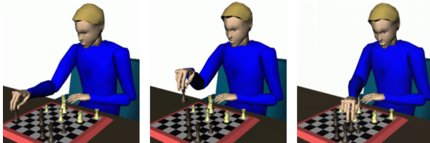
Figure 2.1: 7 DOF arm motion generated by an RRT planner by Kuffner et al. [KL00c]. Copyright 2000 IEEE.
