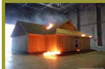
Photo 2. In order to be effective, external sprinklers must be able to wet all areas where ignition can occur, or be sufficiently effective in quenching embers that approach the home so they won't have enough energy to ignite combustible items.
