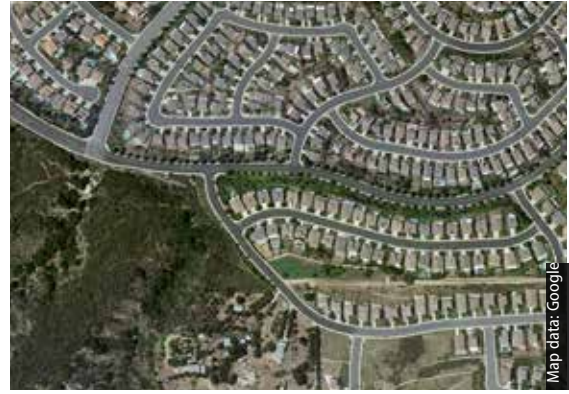
Figure 10. Localized concentration of homes on the inner side of a perimeter road near Alberhill, California. Roads, sidewalks, and yards all become defensible space between the wildlands and structures when homes are sited in this fashion.
