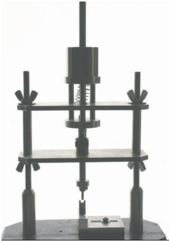
Figure 2. Fracture apparatus. Apparatus used to deliver a highly reproducible fracture injury of DAP12 -/- and B6 mice. The right tibia was centered on the base and a 500g weight was lifted to a distance 3.5 cm. The weight was then dropped to create a closed mid-diaphysis fracture via three-point bending
