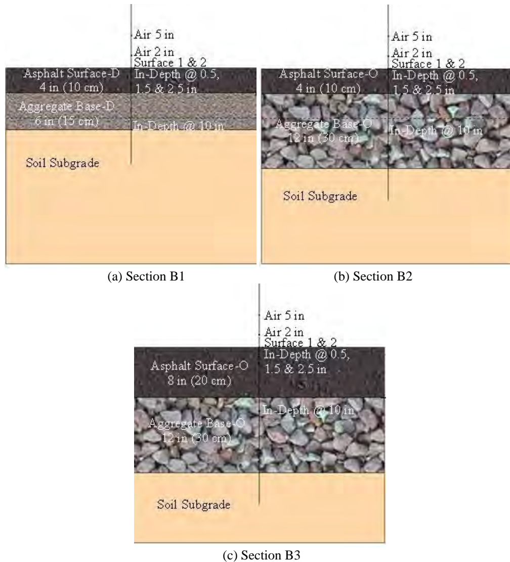
Figure 8.1. Cross sections and sensor locations for the test sections (examples: B1 – B3).
