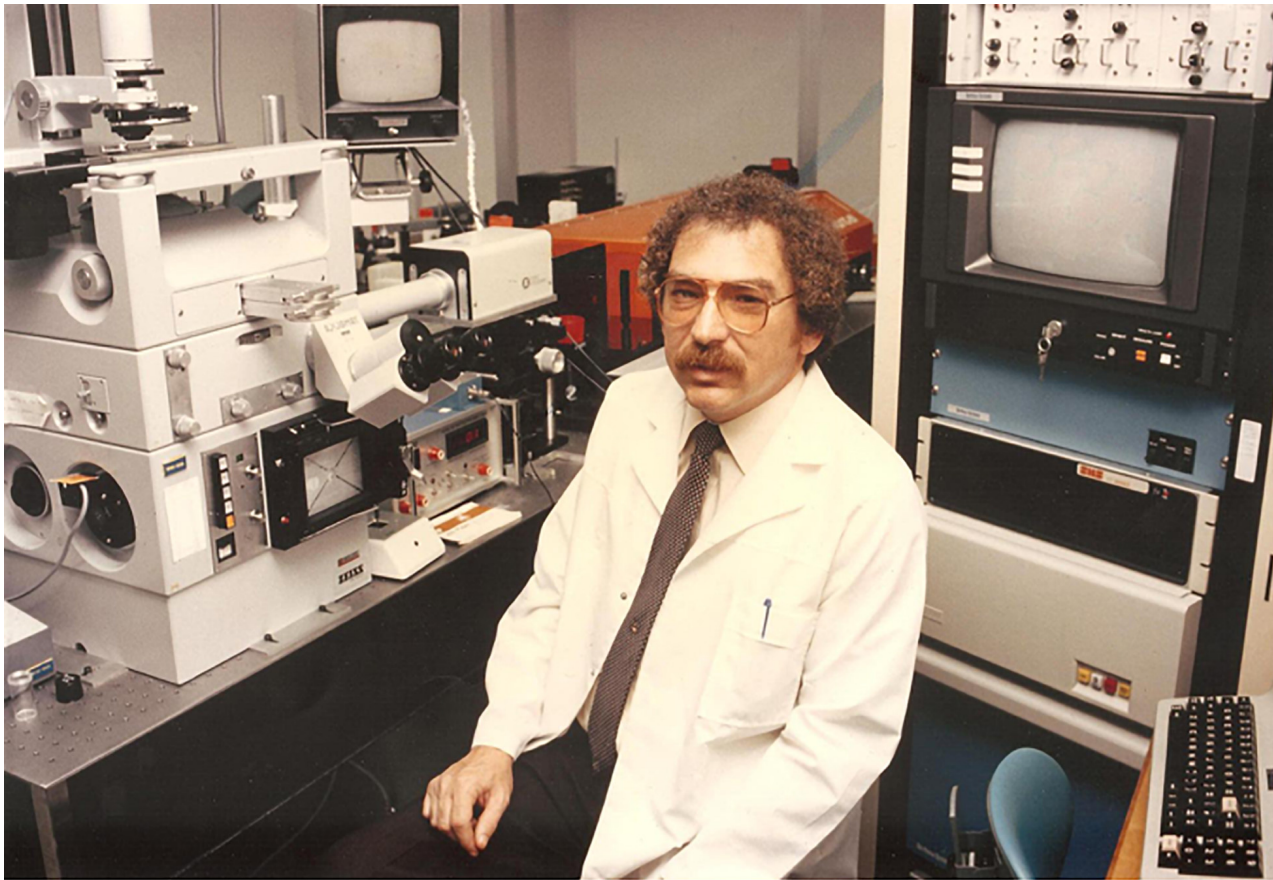
FIGURE 5 | Photograph of system and author circa 1981. The computer behind the PI (principal investigator) is an LSI-11 driven Deanza image array processor. The microscope is a Zeiss Axiovert phase contrast, polarization system. The camera is digital imaging system which signal is sent to the computer system behind the PI. See Figure 4 for details about the system components. This system was used for experiments conducted between 1980 and 2000.
