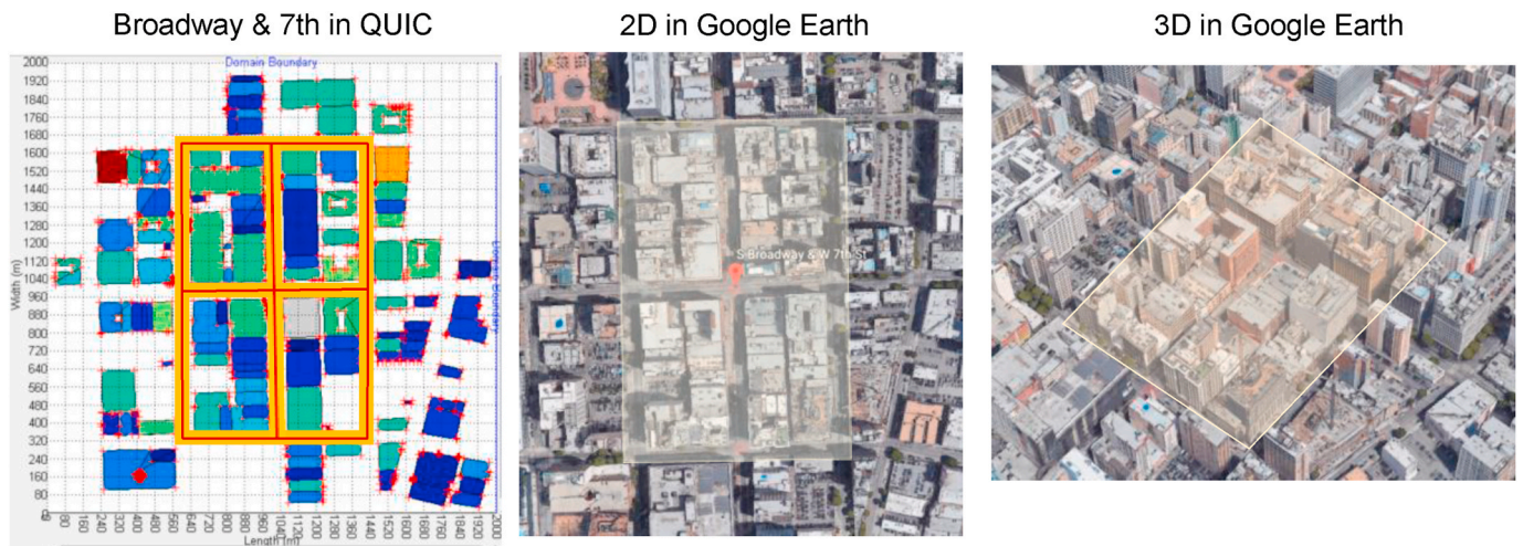
Fig. 1. Building shapes and the QUIC simulation domain in 2D and 3D Google Earth views for the Broadway & 7th site. The yellow bands in QUIC map are the main and sub-main streets and indicate the driving pattern where measurements were collected. Red lines are the line sources from the traffic. Light yellow squares in Google Earth satellite view are the 2 \times 2 blocks we are focusing on. The colors of the buildings from dark blue to red represent the building height from low to high. (For interpretation of the references to color in this figure legend, the reader is referred to the Web version of this article.)
