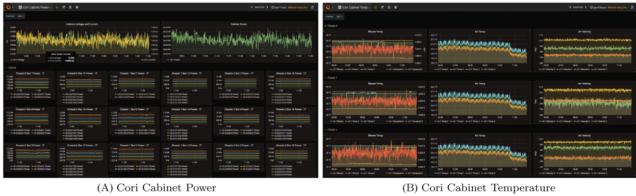
FIGURE 2 Screenshots of Cori telemetry Grafana dashboard showing (A) cabinet power and (B) cabinet temperature
