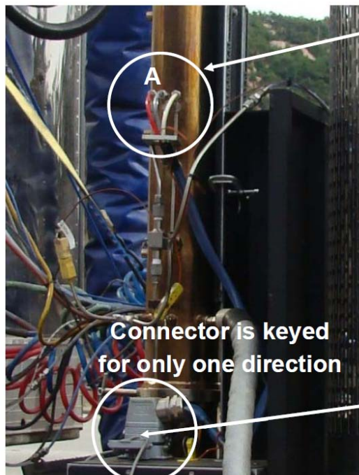
Figure 6-20 PEMS2 exhaust flow connection between units1 compared to units 2 and 3
