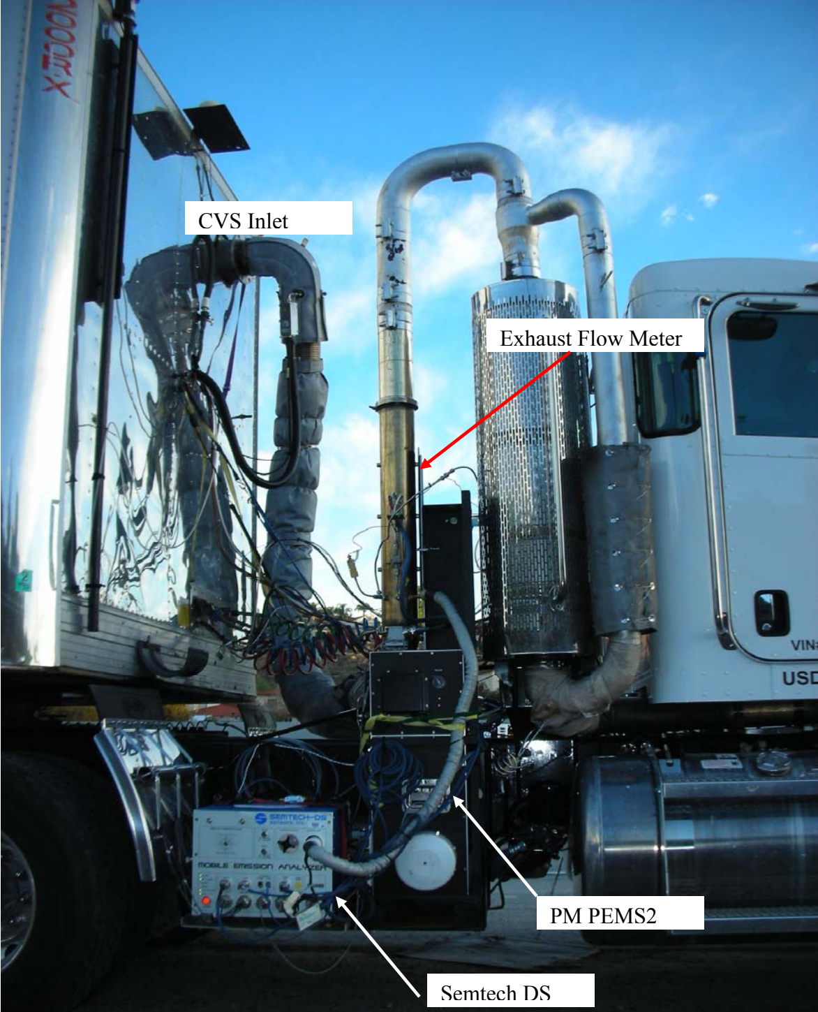
Figure 3-6. PEMS2 installation with Semtech DS system: passenger side on frame
