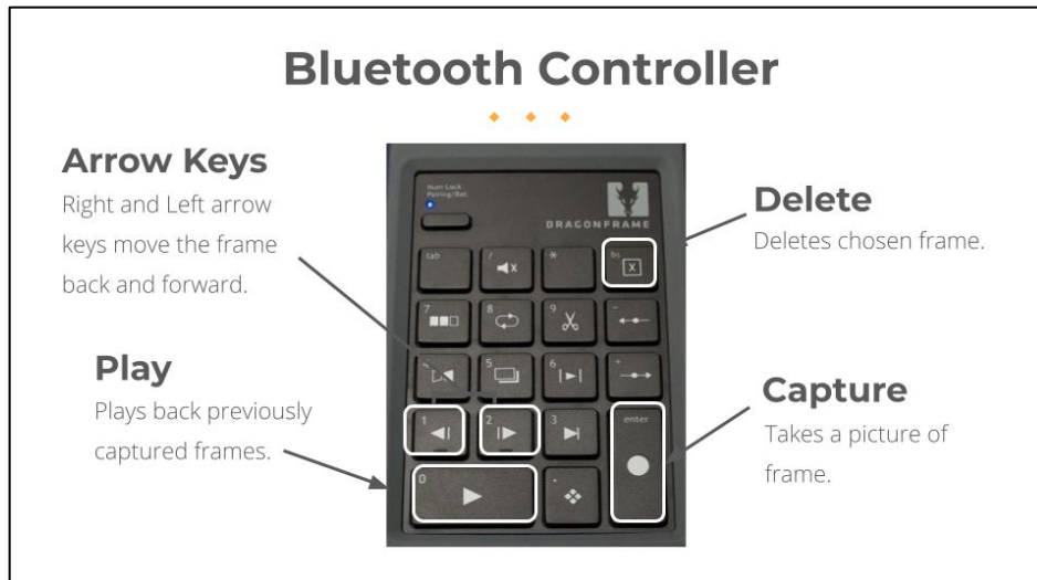
Figure 4.3. The wireless Bluetooth keypad provided by Dragonframe. In our study, subjects only needed to use the five buttons outlined in white to CAPTURE (photograph) a frame, to DELETE one or more frames, to use ARROW KEYS to move around among already-captured frames, and to PLAY, that is, view, all the frames they already captured.
