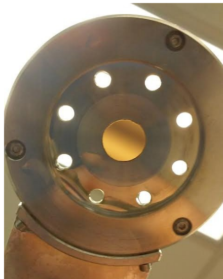
Figure 4.2: Aluminum frame with 40 \mu\text{g}/\text{cm}^2 carbon foil mounted. This frame inserts into the center of the copper detector body.
