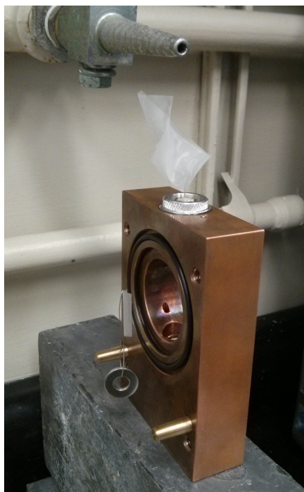
Figure 4.5: Anode wire placement: a small weight is used to apply tension on the wire while epoxy is applied and allowed to cure.
