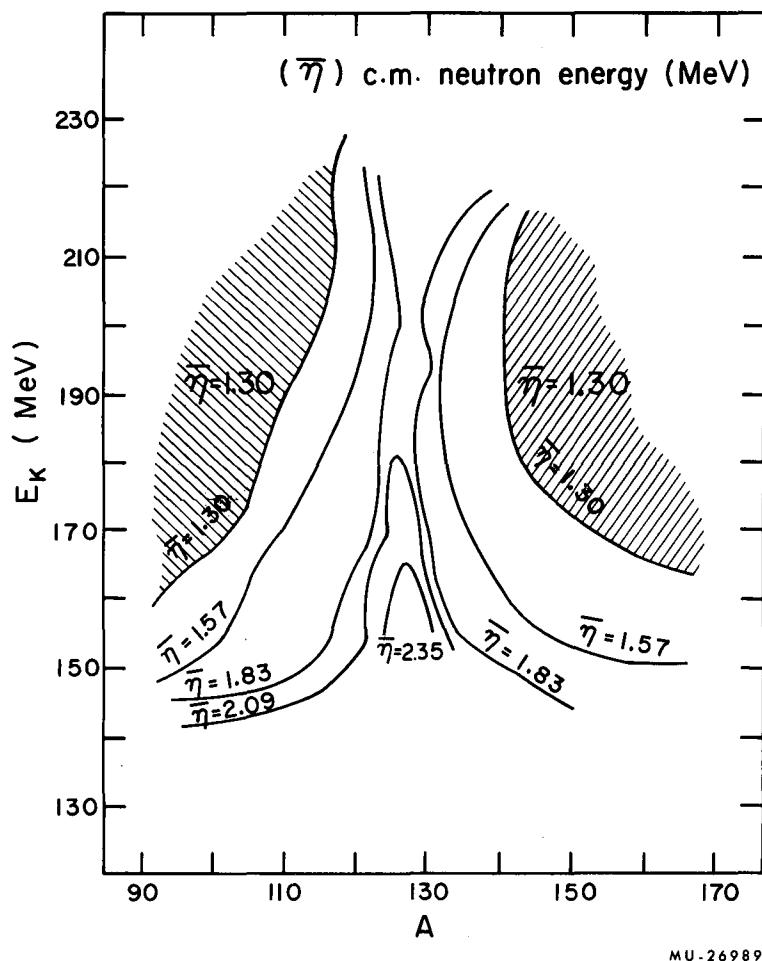
Fig. 4B. Contour diagram of the center-of-mass neutron kinetic energy  $\bar{\eta}$  as a function of fission fragment mass  $A$  and total kinetic energy  $E_K$ . The contour lines are lines of constant neutron kinetic energy. ( $\bar{\eta}$  is constant over shaded areas.)
