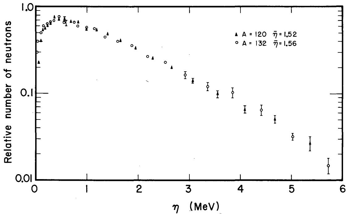
Fig. 17. The relative center-of-mass neutron energy distributions, proportional to  $\phi(\eta)$ , corresponding to neutrons coming from mass 120 and from mass 132.
