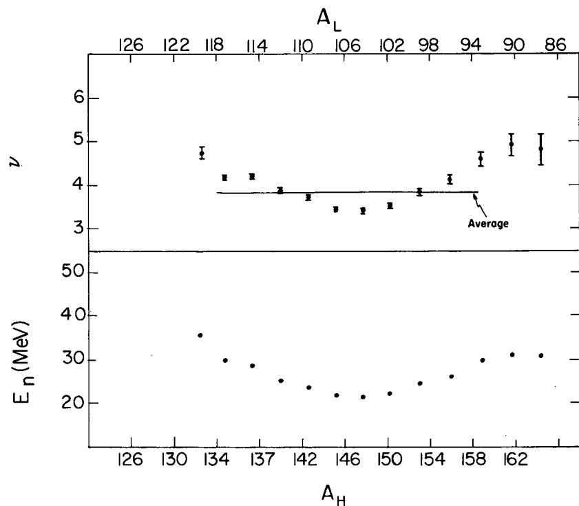
Fig. 11. Total number of neutrons per fission  $\nu$  and total energy  $E_n$  in the form of prompt neutrons as a function of mass pairs.
