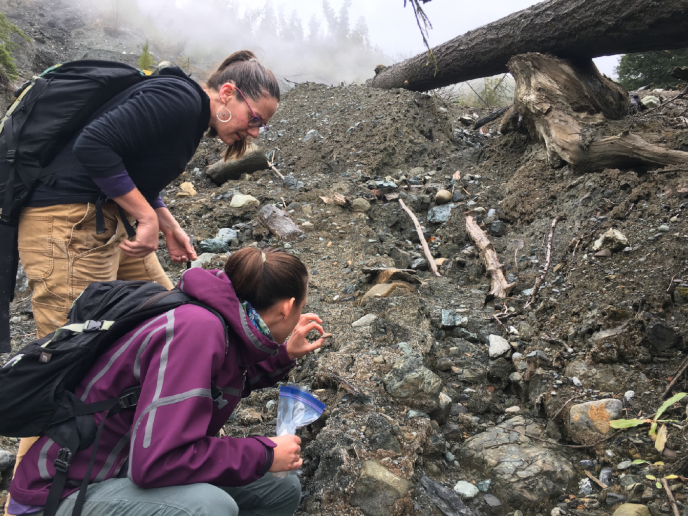
FIGURE 18.2.7 Lawrence Livermore National Laboratory scientists examine ultramafic rocks in Washington state. These rocks are rapidly reacting with \text{CO}_2 and breaking down to calcium and bicarbonate ions, leaving clays and unreacted blocks of rock behind. This site is a landslide—as the rocks break down, they lose structural integrity and slide downhill. Photograph by Roger Aines.
