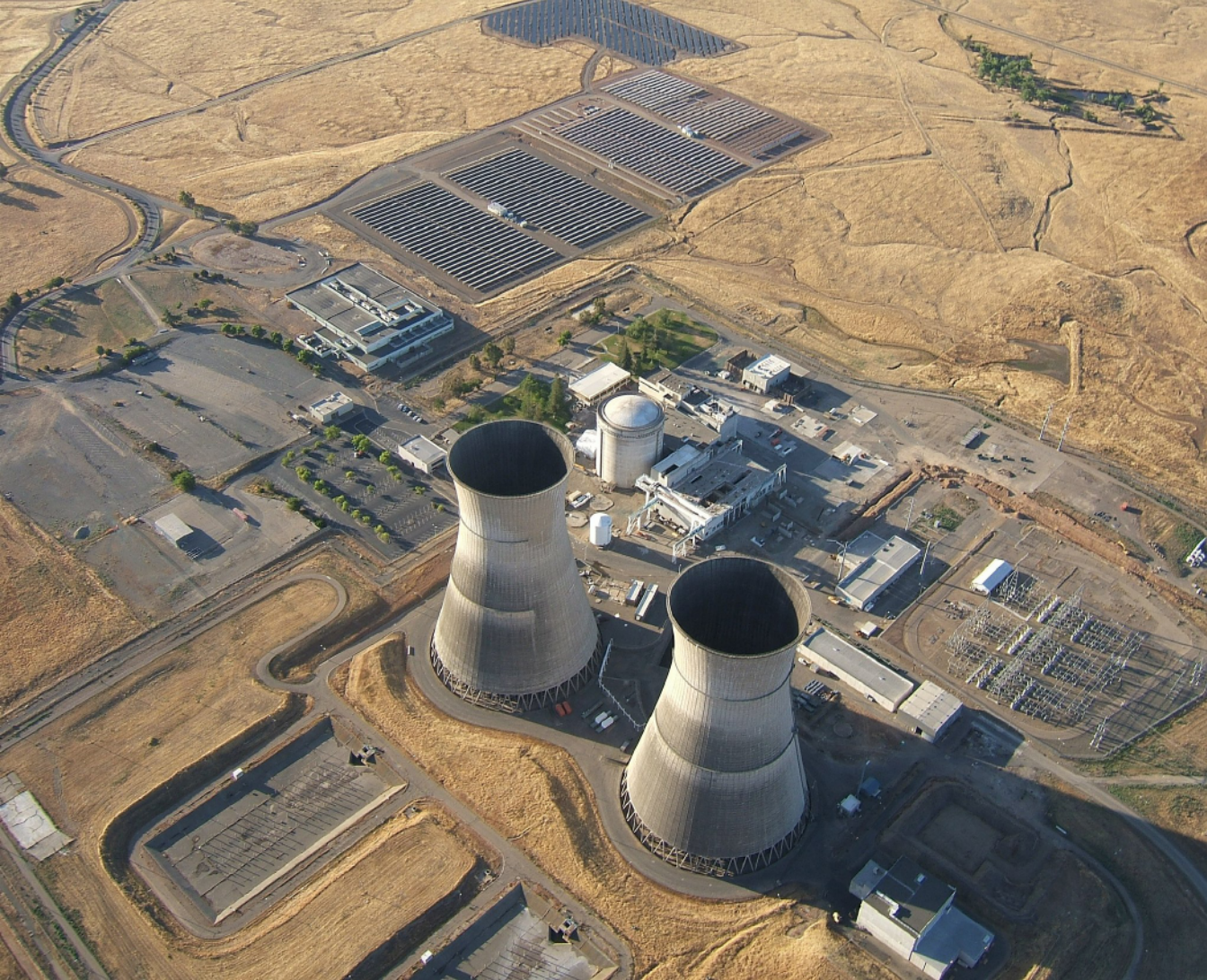
FIGURE 9.4.3 Rancho Seco. The decommissioned Rancho Seco nuclear power plant in Sacramento County now hosts a solar farm and is under contract to the Golden 1 Center, the home of the Sacramento Kings. At full build-out, the facility will provide up to 100 MW of power, taking advantage of the transmission lines and other infrastructure built for the nuclear plant. Photograph by Hajhouse from Wikimedia Commons.
