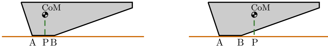
(a) A statically stable object. Static stability margin is given by \min(PA, PB) , the minimum distance from P to the edges of the support polygon. (b) A statically unstable object. Static stability margin is given by -PB , minus the minimum distance from P to the edges of the support polygon.
