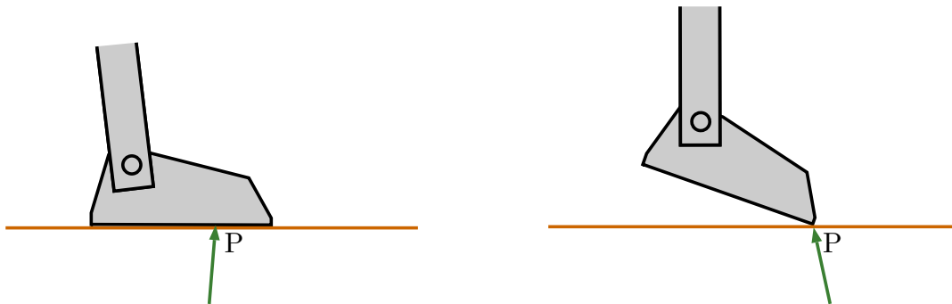
(a) ZMP criterion is met (center of pressure is strictly within footprint). As a result, the foot does not rotate. (b) The foot is rotated and the robot touches the ground only at a point. Then this point is where the ZMP acts.
