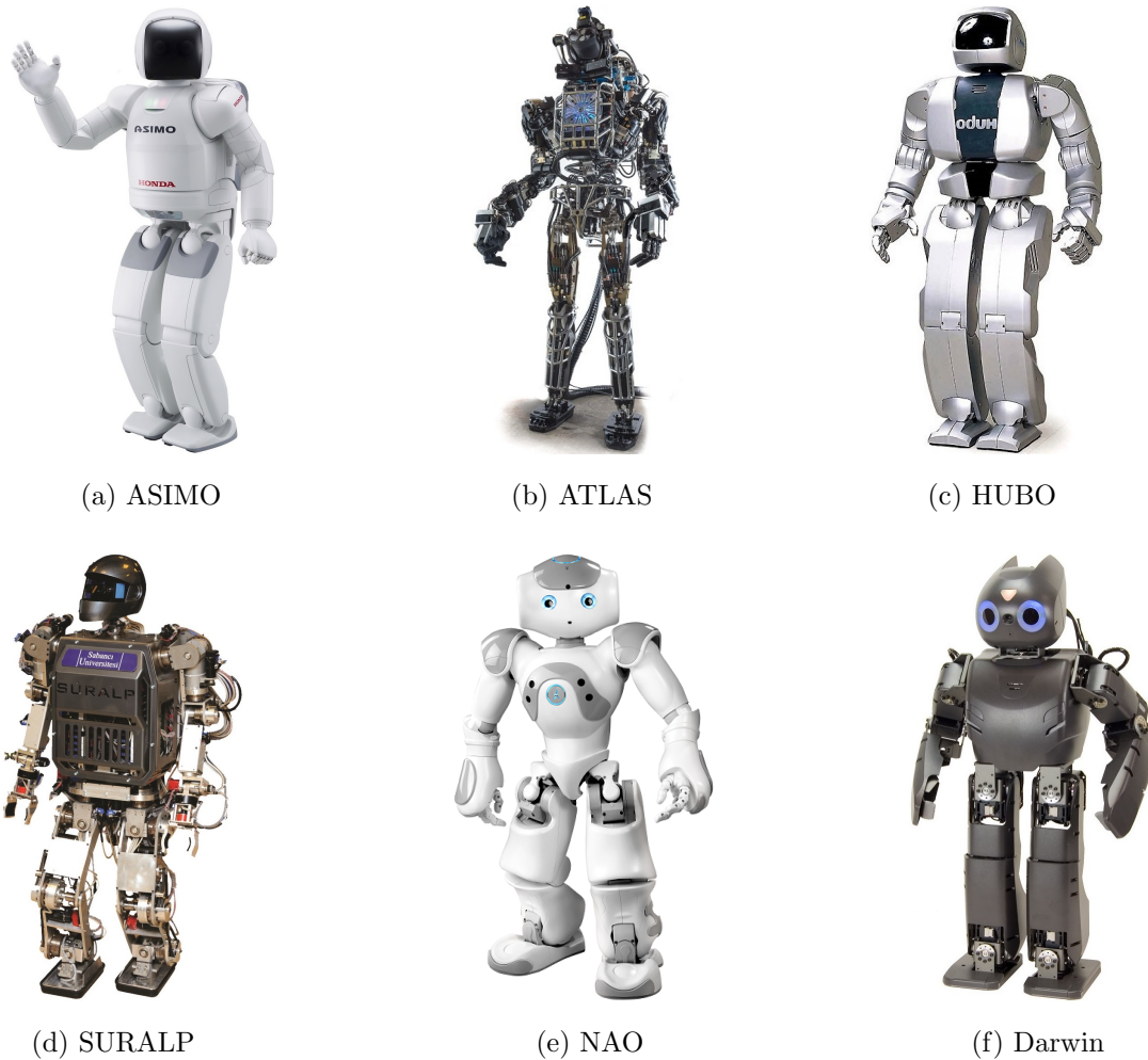
Figure 1.1: Some state-of-the-art bipedal robots with large feet. ASIMO, ATLAS, HUBO and SURALP are human sized robots built for research purposes. NAO and Darwin are smaller bipeds which are commercially available.
