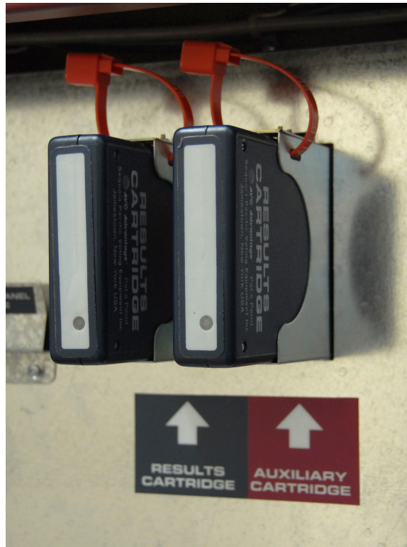
Figure 2.6. The machine has slots for two memory cartridges. The first cartridge stores ballots and votes. An attacker could install vote sealing code by inserting a prepared cartridge into the second slot.
