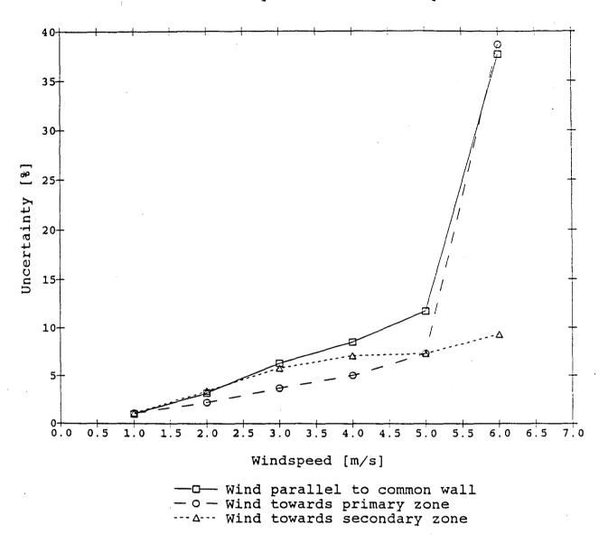
Figure 1. Uncertainty (scatter) in the measured leakage coefficient of the common wall between two apartments as a function of windspeed for three different wind directions (based upon reference simulation).
