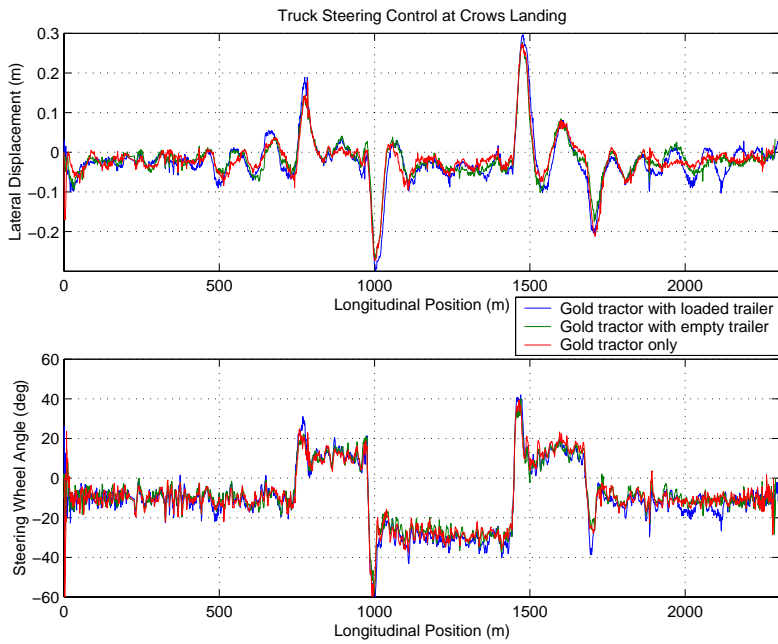
Figure 4.5.6: Speed and steering angle for tractor semi-trailer (with 5000 kg load) and FDL120 tractor only configuration (along longitudinal position at the track)
